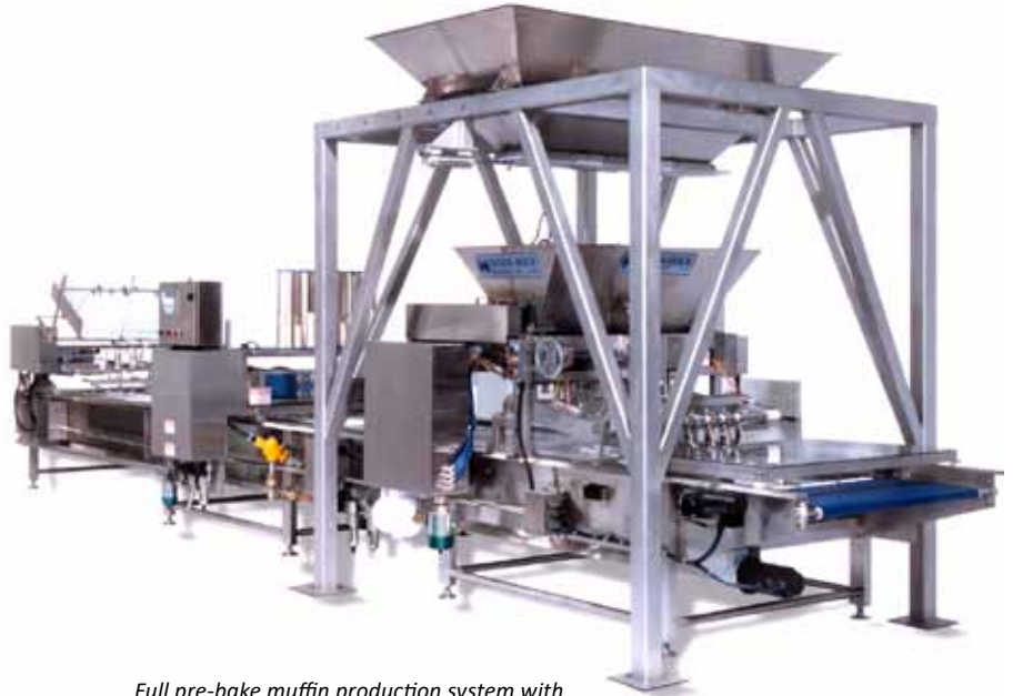
Full pre-bake muffin production system with paper cup denester and multi-piston depositor.
