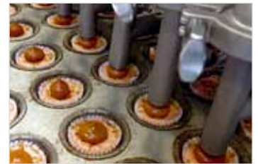
Fully automated multi-piston bakery production system with cup denester, crumb depositor, tamper and toppings depositor.
