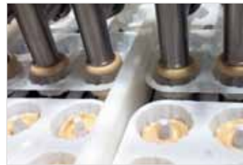
Fully automated multi-piston bakery production system with cup denester, crumb depositor, tamper and toppings depositor.
